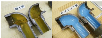
Cleans the inside of the piping and lasts longer due to lining processing
